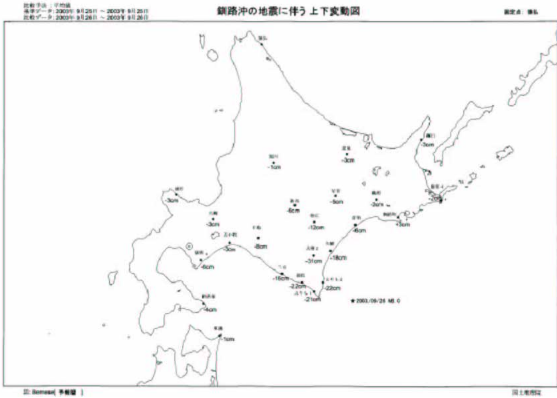
Figure- 20. Vertical Movement during 2003 Tokachi-oki Earthquake Obtained from GPS Observation by GSI
