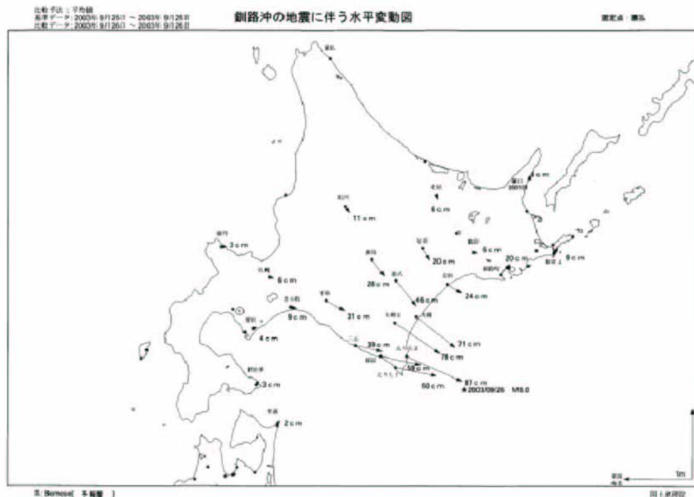
Figure-19 . Horizontal Movement during 2003 Tokachi-oki Earthquake Obtained from GPS Observation by GSI
